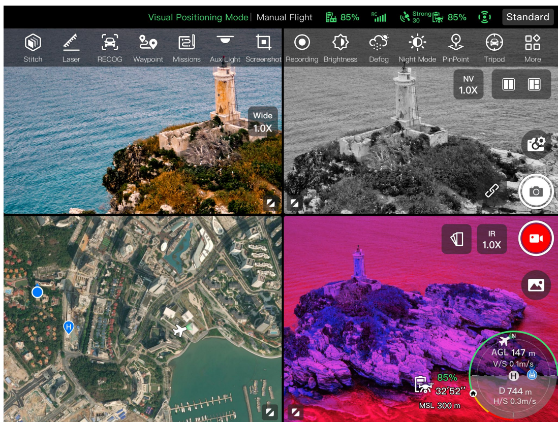
Fig 6-3 Display of the Autel Enterprise App in Four-Screen Mode (Fusion 4N Gimbal)
